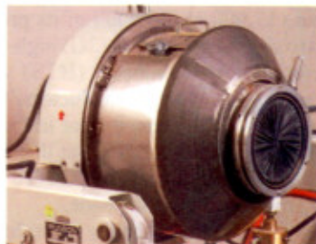
Miniature rotary batch mixer with loading port and iris valve closed, ready for a mixing cycle.
