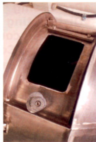
Munson MX-1-SSJ miniature rotary batch mixer with mixing vessel jacket plumbed to a water-heating unit (above); Loading port of the miniature rotary batch mixer (right).
