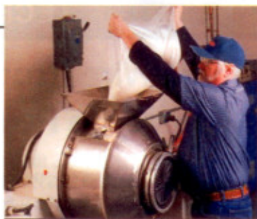
General Cable technician loads pelletized resin into miniature rotary batch mixer.
