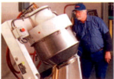
Technician tilts the mixer to vertical for discharging.
